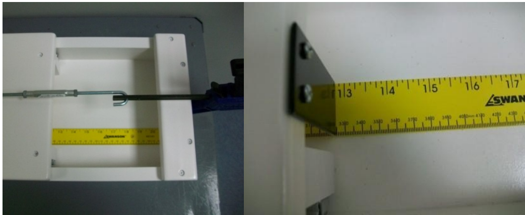
Figure 13 & 14 Reading the Ruler on the Panty Sizing Device to the nearest ½ inch
